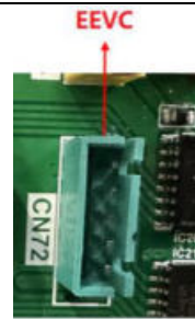
Figure 1 Main board port
