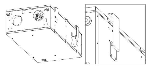
4. Place 4 hinge locks on joints of mounting brackets.
